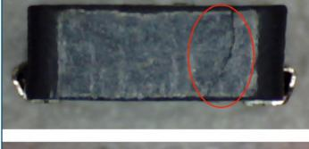
Lateral crack: Crack covers more than 50 % of the length of the side.
