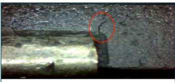
Crack around soldering pad that does not extend to the top or side edge.
