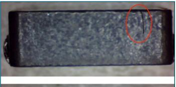
Vertical crack: Crack does not extend from one side to another.
