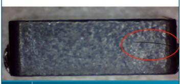
Lateral crack: Crack covers less than 50 % of the length of the side.
