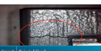
Figure 8 Rejected Crack
