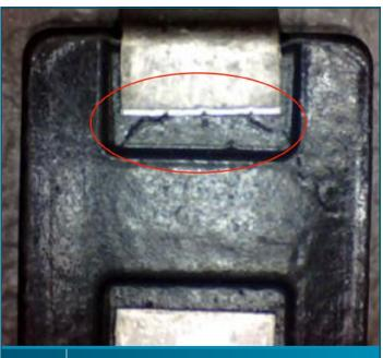
Crack is located only at the groove of the body and does not extend beyond convexity.
